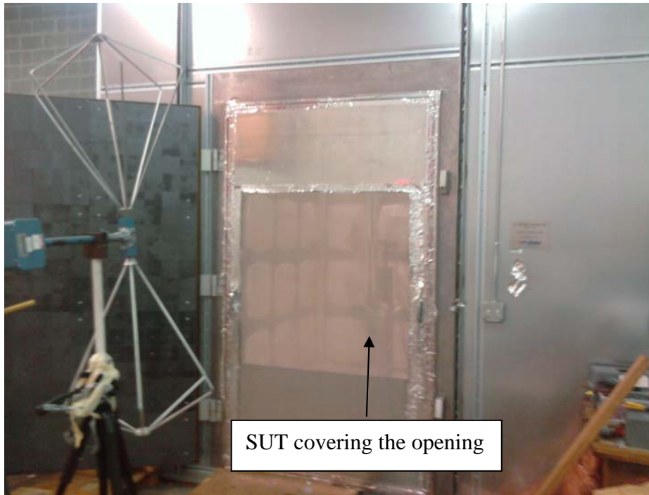
Figure 5. High Frequency (100 - 200 MHz) Test Configuration Photograph
